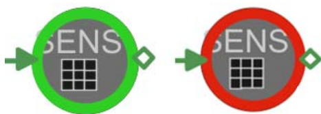
Figure 5 Icons of sensor (“SENS”) models on the flowsheet in PSE’s hybrid modelling tool turn red when model quality criteria are not met.
