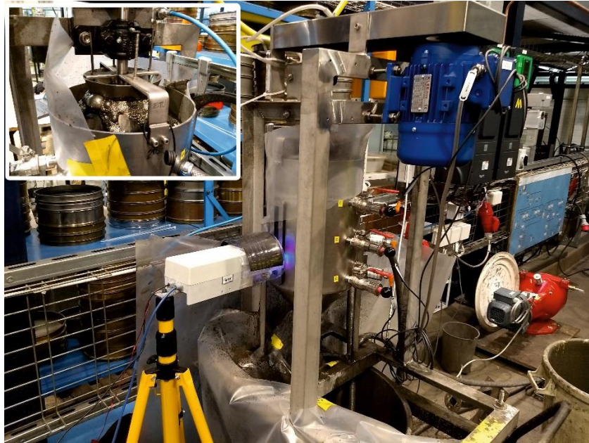
Figure 2. Coarse flotation device in minipilot-scale. On top, a copper concentrate is flowing from the top of the device. In the lower left corner, the particle tracking measurement device is also seen.
