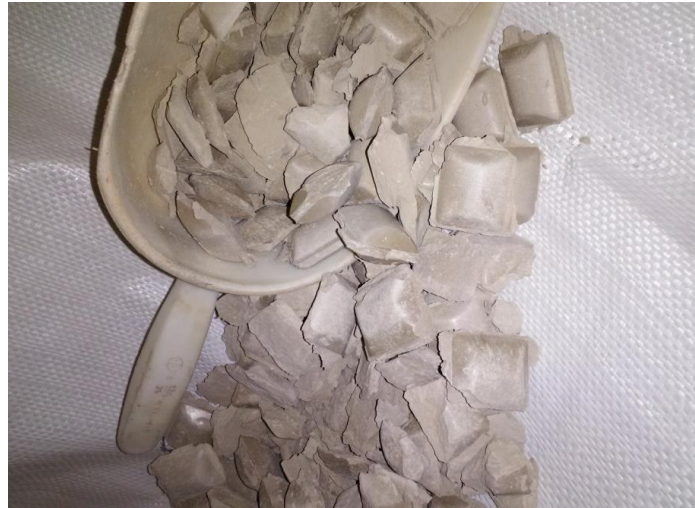
Figure 4. Pelletized material resulting from the rolling compaction stage of the Manfredini Fusion system.
