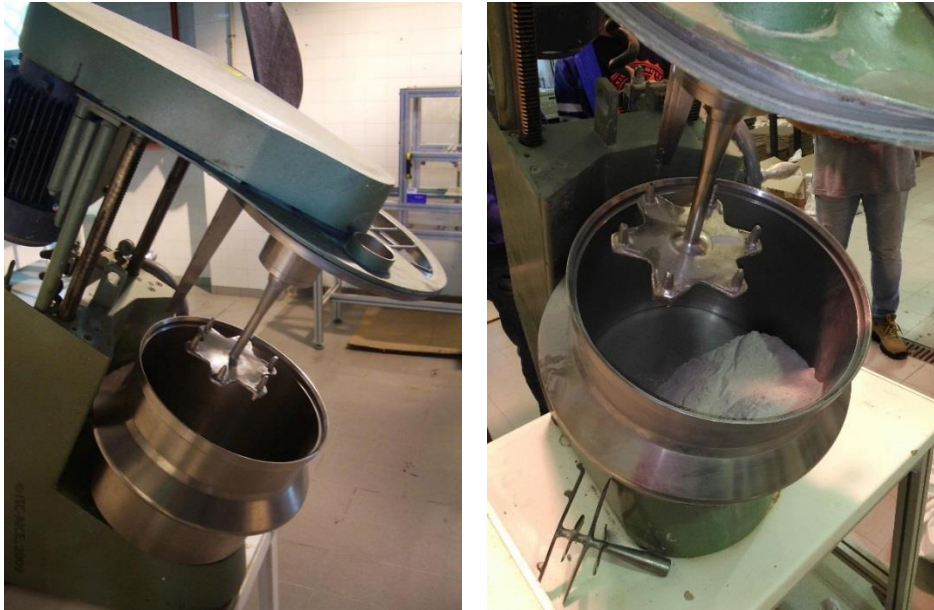
Figure 6. High shear mixing equipment.
